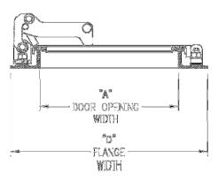
The Quick Opening Access Door is designed to be field mounted to any existing flat surfaced vessel. Field cut an opening in the vessel based on the door opening width "A" and the mounting opening height "B". The door can then be welded or bolted in place using the integral mounting flange
