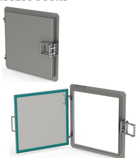
Our Quick Opening Access Doors are designed to be mounted on any flat vessel and can be bolted or welded in place at installation. These doors provide quick opening tool free access with a tight positive gasket seal.
