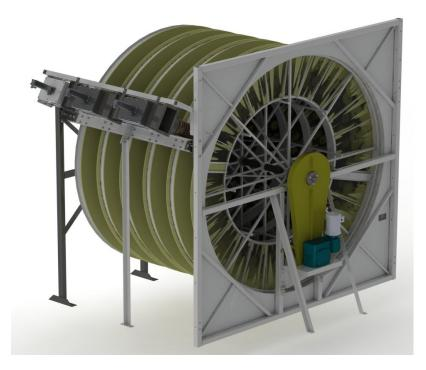
The Circle Vee Drum Filter is a revolutionary concept in air filtration. With its unique design, the Circle Vee can be installed in a fraction of the space required for conventional systems. The stationary nozzles clean both sides of the media as the Circle Vee rotates. The stripper fan cleans fine dust and other materials from the filter media making the Circle Vee completely self cleaning. Clean media assures a uniform pressure throughout the system.
