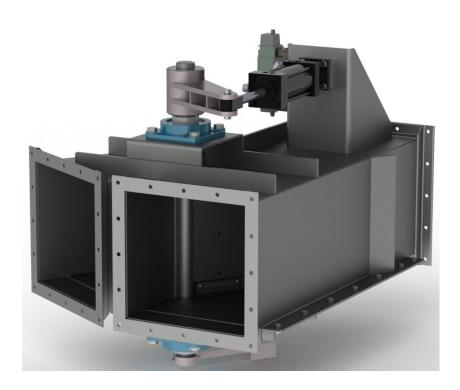
Our diverters are designed to handle applications where there is dust or fiber loading in the air stream. The pneumatic actuator provides full stroke blade positioning, diverting air from one side to the other. Typical applications include diverting air from on-line hoods to an air bleed to maintain conveying velocity in the duct network in the event of a sheet break or thread-up operation.
